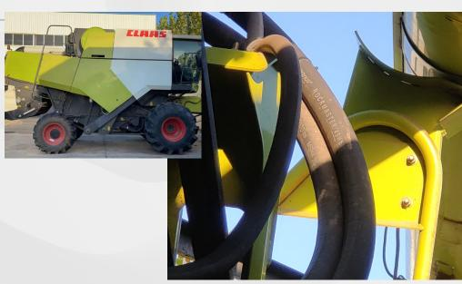
MH ROCKMASTER/4SH hoses on CLAAS machine made in China
