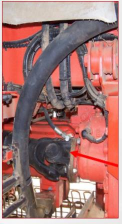
Severe heavy duty hose application on hydrostatic drive:
