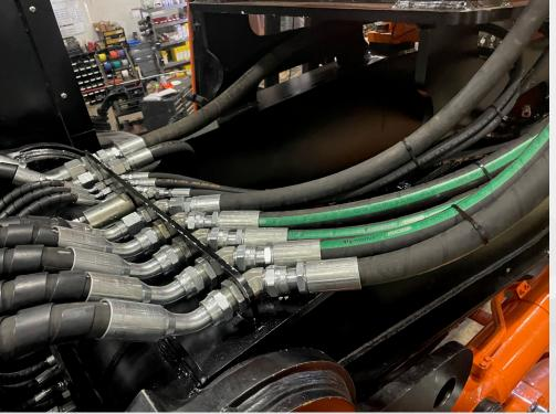
Special machines and attachments for forestry applications (USA). ANACONDA hose is selected for its high flexibility and suitability in difficult installations.
