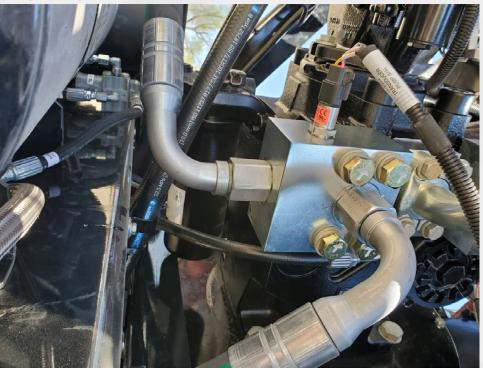
**CNH (USA)** approved and put in manufacturing drawings the MH **Fast-Fit**, here relevant photos, with ANACONDA hose (420 bar) and Zinc-Nickel technology (e-coat 1000). Restricted spaces for installation and easier maintenance.
